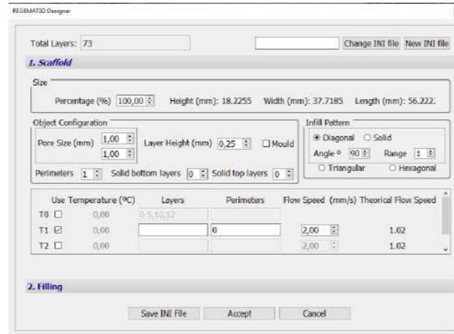
2. Facilitates the configuration of different parameters: layer height, pore size, perimeters, type of infill, etc.
